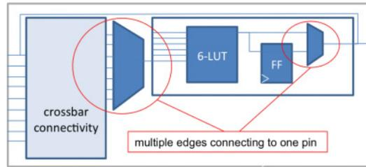
Fig. 3. MUX inference within a logic block.
