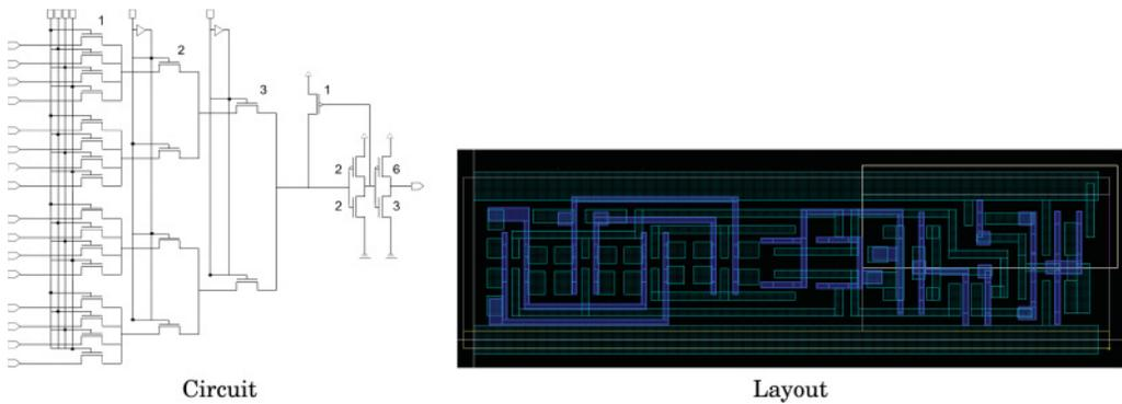
Fig. 11. MUX16 transistor-level circuit and custom layout.
