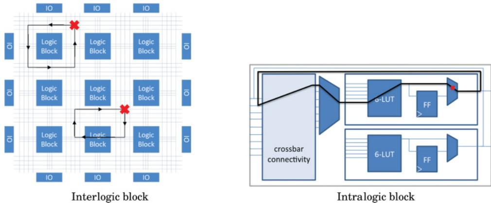
Fig. 6. Breaking combinational loops in routing.
