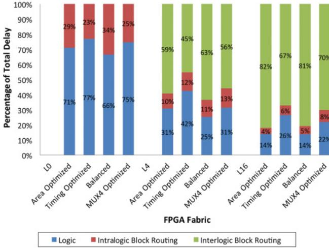
Fig. 10. Delay breakdown.
