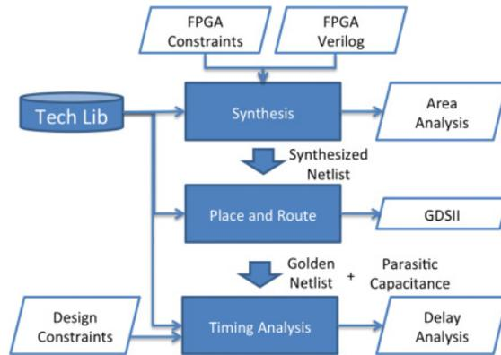
Fig. 5. ASIC design flow.
