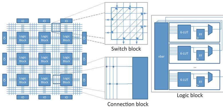
Fig. 2. FPGA architectural components.
