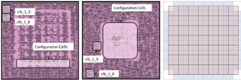
Fig. 7. Floorplanned (left) and unfloorplanned (center) layout and floorplan grid (right).
