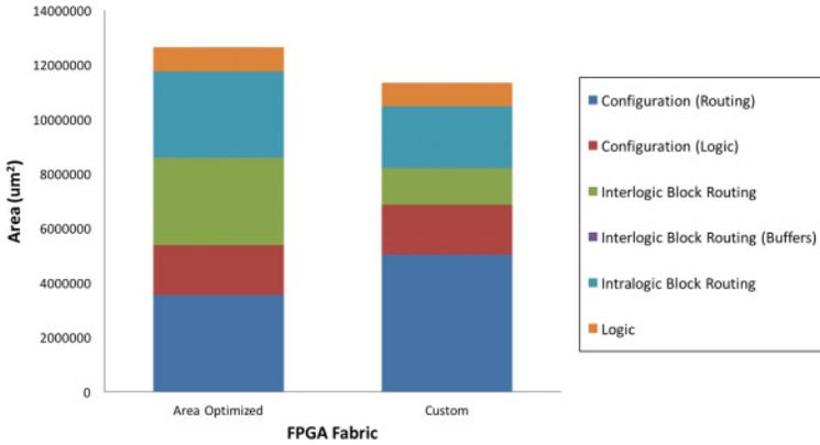
Fig. 12. Area breakdown of an area-optimized FPGA and an area-optimized FPGA with a custom cell.
