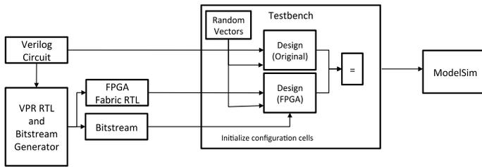
Fig. 4. Synthesizable FPGA verification flow.
